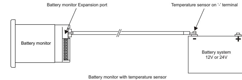
Battery monitor with temperature sensor
