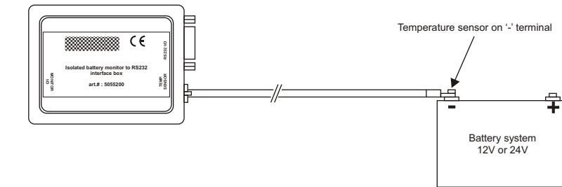
Isolated interface box with temperature sensor
